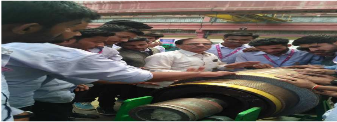
Mr. Chaudhari explaining dc motor armature
